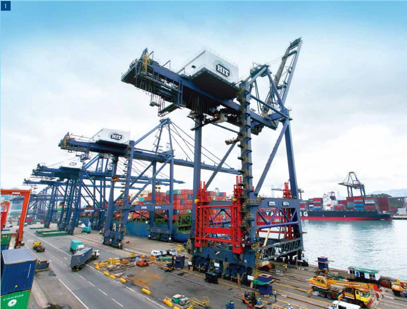
1. The jacking frame (in red) heightens Quay Cranes at HIT by three metres.
